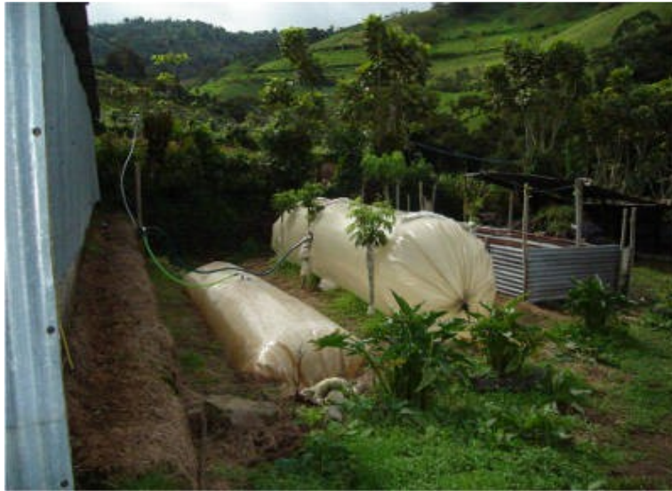
Fig. 6 : A locally manufactured biodigester with a low cost polyethylene tube in Costa Rica (source redbiolac.org)
