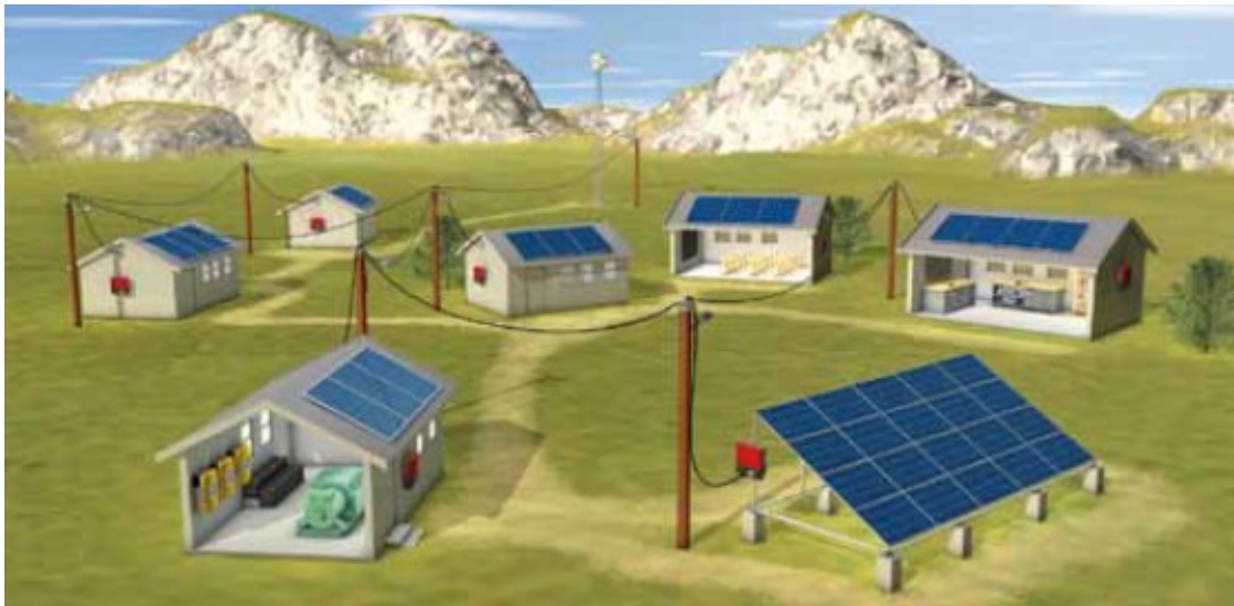
Fig. 9: A rural microgrid (Source: www.sma.de )
