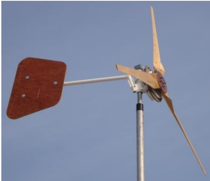
Fig. 4 : A locally manufactured small wind turbine following the design manuals of Hugh Piggott (Source: www.rurerg.net )
